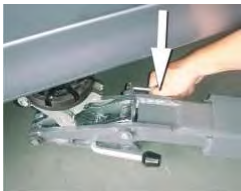
Figure 3: To release the fixture plate, the rear lever must be pushed.
