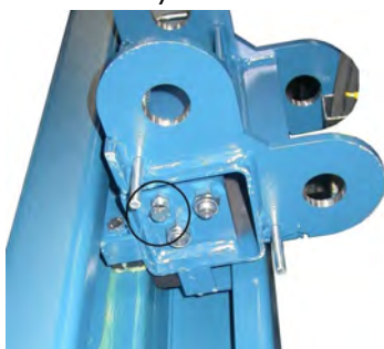
Position of the setting screws
