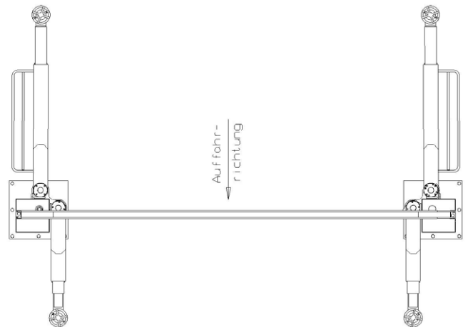
Lifting arm start position Once the lift is in the lowest position, swing out the lifting arms to the start position.
